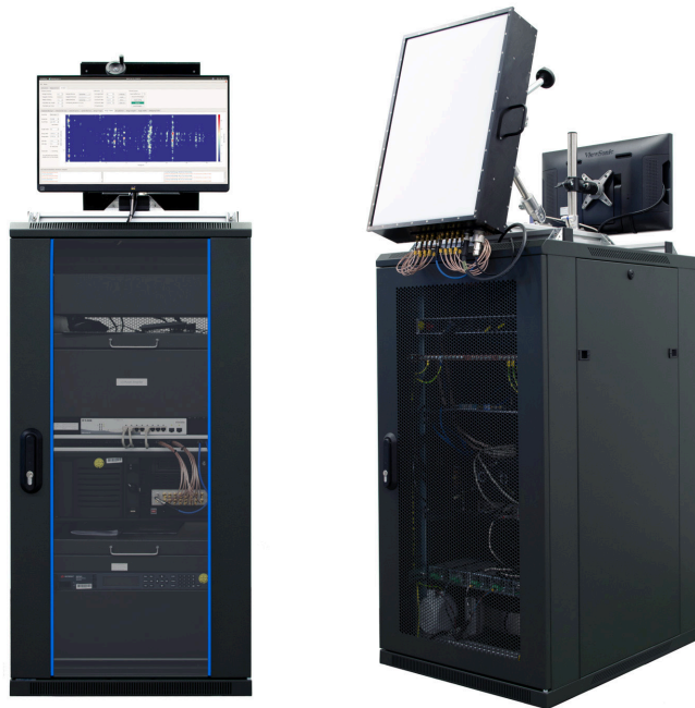
Figure 3: Photograph of the realized demonstrator in a mobile rack. On the top, the RF frontend and the user interface can be seen.
